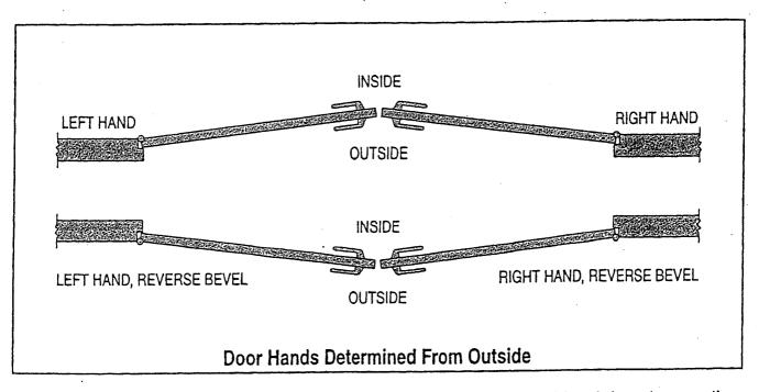
The door handing (left or right) is determined from exterior or outside of door (secure/key side). Exterior and interior handles are defined as follows:
